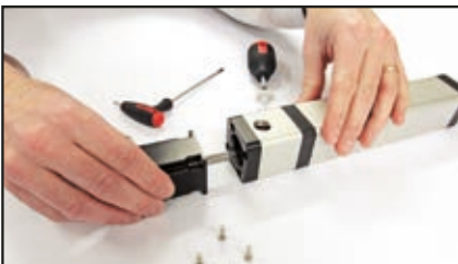
Insert motor shaft into coupling
