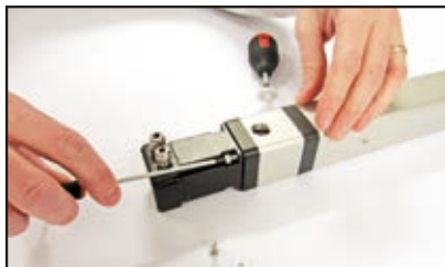
Tighten motor mounting screws
