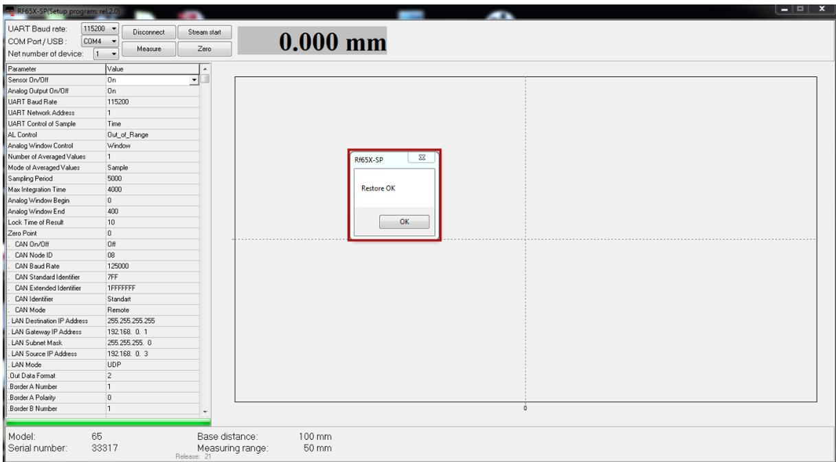
In order for the changes to take effect, you must end the connection session and reboot the micrometer by turning OFF/ON the power supply.
