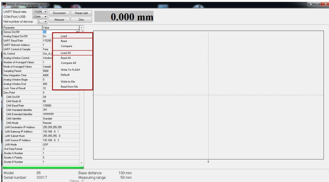
In the pop-up window there are two items: **Write To FLASH** and **Default**. The **Write To FLASH** item allows to save the current parameters from the RAM of micrometer to the non-volatile memory. The **Default** item allows to restore factory settings of the micrometer.
