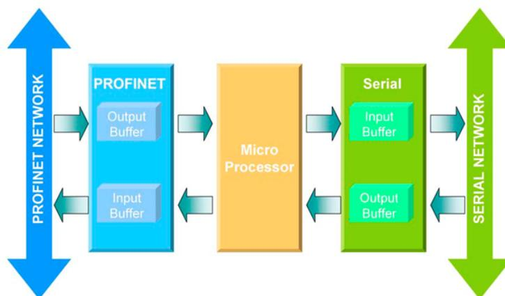
During each message cycle, the PROFINET IO controller writes the content of its output buffer to the PROFINET IO device input buffer and reads the content of the PROFINET IO device output buffer to its input buffer. The exchange cycle is taking place even though the content of the PROFINET IO controller and PROFINET IO device output buffer has not changed. The data flow between the PROFINET IO controller and the I-7580 module is shown below.
