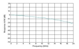
Responsivity measurement of an 80 µm photodiode using the LWP probe and the Agilent Technologies 83420A Lightwave Test Set.
