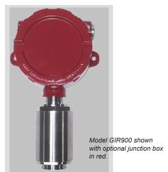
The SST Model GIR900 Infrared Combustible Gas Sensor is a completely self-contained device that measures the concentration of hydrocarbon gas accumulated in a protected area and transmits this information to a central point.
