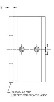
Material: 101mm Bore - Anodized Aluminum 127mm & 152mm Bore - Zinc Plated Steel
