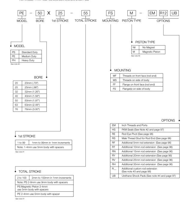
Note 1 - All models use a 5mm stroke body length for 1st Stroke of 5mm or less. 1st Strokes over 5mm use body length of the actual stroke + adder.
