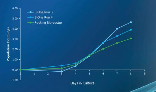
**Cell Culture**. Growth profiles and titer were evaluated with a CHO cell line in a 17 day fed-batch process. Titer was quantified starting on Day 6. Similar growth and titer were observed in the BIOne and glass vessel control. Performance results indicate that the BIOne single-use bioreactor system is a suitable bench scale SUB for mammalian cell growth and recombinant protein production.
