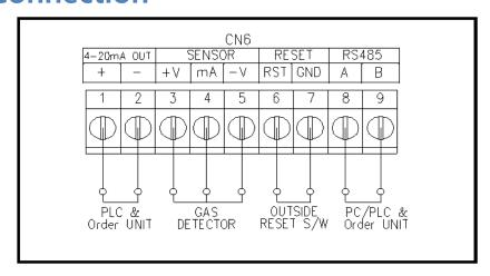
Caution) RS-485 Cable should be used dedicated RS-485 cable and for the connection cable to connect with 4~20mA output and detector, the shield cable of CVVS or CVVSB higher than 0.75sq should be used!
