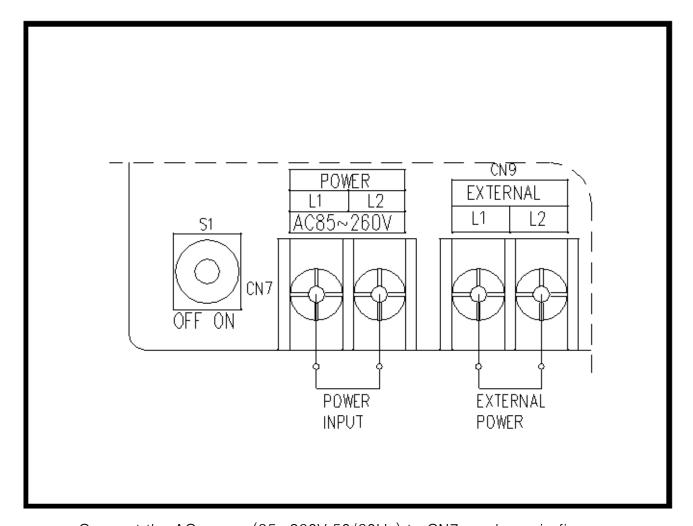
Connect the AC power (85~260V 50/60Hz) to CN7 as shown in figure.
