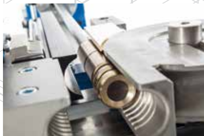
Mandrel bending tool with ball-type mandrel
