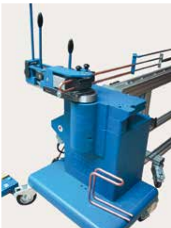
Mandrel bending machine 4800 with special tool
