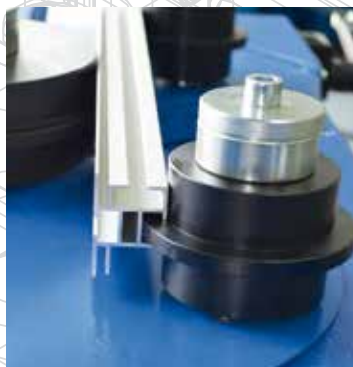
Section tube with special tool on RB60
