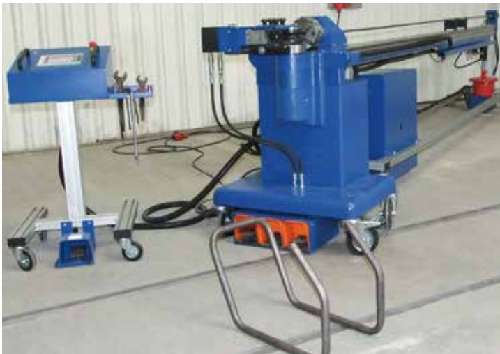
Retrofit to right/left bending enables bending of symmetrical bending workpieces
