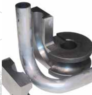
Mandrel bending tool bend-to-bend (e.g. door handle)
