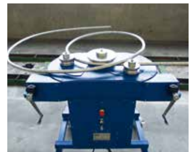
Spiral on 3-roll bending machine RB60
