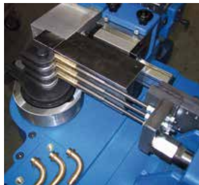
Special construction mandrel bending device 5000 with 3-fold bending tool
