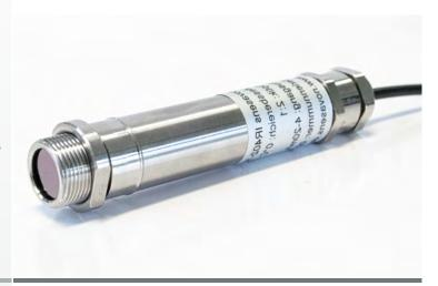
The novasens IR402 infrared temperature sensor measures temperatures from -20°C to 250°C without contact and is equipped with a thermocouple output of type J or K or analog output 4-20 mA.
