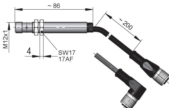
The limit switch can be used to monitor minima or maxima.
