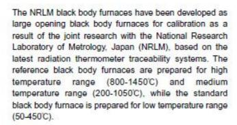
The black body furnace for high temperature is used for comparison calibration by using a fixed-point-calibration by using a fixed-point calibrated 0.90 or 0.65 µm silicon monochromatic radiation thermometer as the standard thermometer.
