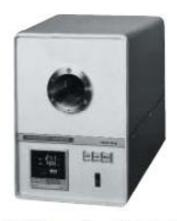
The black body furnace for medium temperature range is used for comparison calibration by utilizing a fixed-point calibrated 0.90 µm silicon monochromatic radiation thermometer as the standard thermometer, and the black body furnace for low temperature is used for calibration by utilizing a optional built-in platinum resistance thermometer as the standard thermometer.
