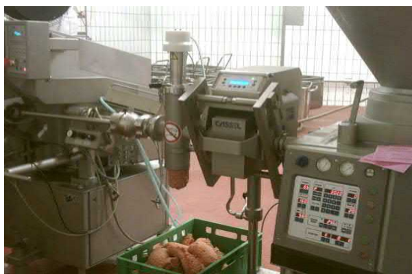
METAL SHARK® IN Meat fitted into a production line.
