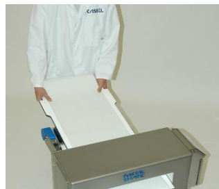
Pull the PU belt as well as the sliding plate out of the unit.
