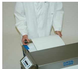
Now you can easily remove the Pulley from its guide.
