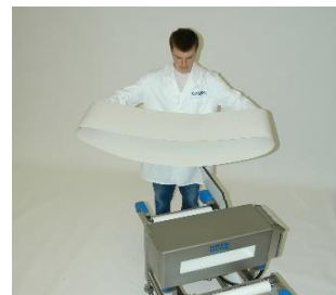
Remove the PU belt completely from the sliding plate.
