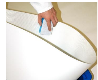
Clean PU belt with a sponge or the hose. Use soap and water.
