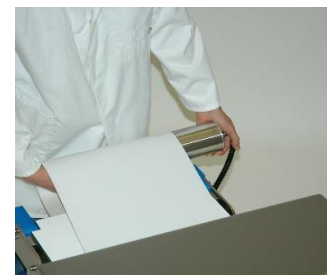
Go to the other side of the conveyor and remove the deflection roller there.
