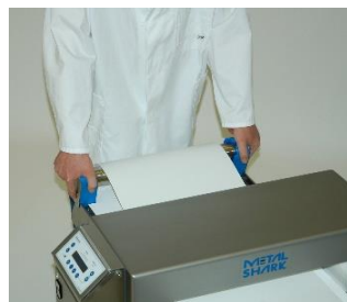
Fold the guide of the deflection roller upwards.
