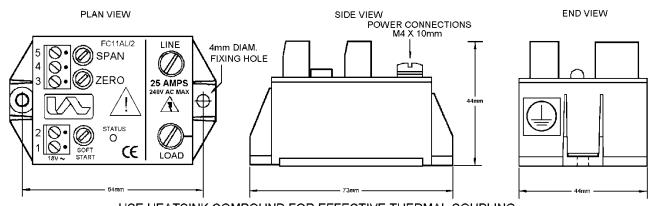
USE HEATSINK COMPOUND FOR EFFECTIVE THERMAL COUPLING WARNING LIVE TERMINALS
