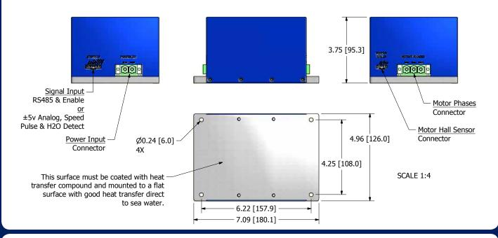
Download STP solid model of this electronics module here: http://www.tecnadyne.com/thrusters
