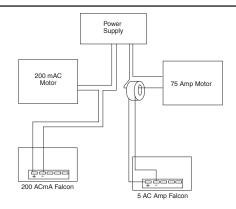
jumper from DPC to DP3 on rear terminal block. Next remove the front bezel. Adjust potentiometer VR101 until the display indicates 75.0 (amps) when the 5 amp signal is ON. Replace the bezel, and remove the signal.
