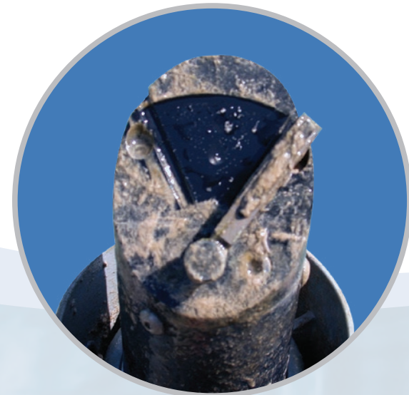
Despite significant bio-fouling after a 12 month deployment, the optical face of the DTS-12 is clean and perfectly operational.
