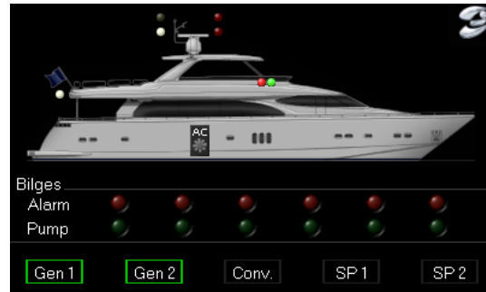
Page 1: navigation lights status, bilge level alarms, bilge pump status, generator status
