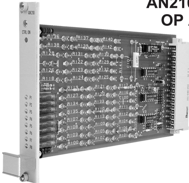
**The AN 210 module has been designed as a logical element for systems. The many different OP circuits, solder tags for components and the possibility of external interconnection for the individual OP amplifiers make this module suitable for a wide range of applications.**
