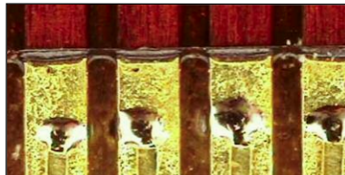
Welding 0.008 in thick copper terminals
