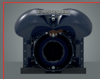
New high efficiency reversing bucket and steering nozzle design
