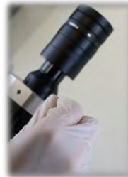
6 Screw the optical head
