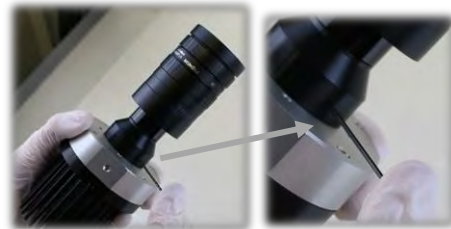
4 Unscrew the optical head
