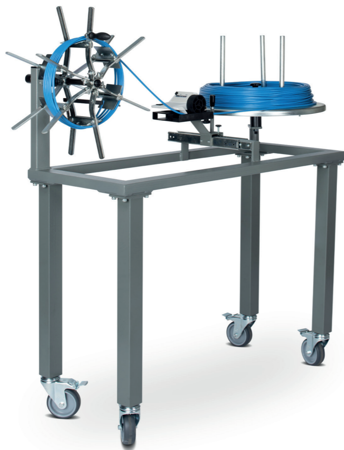
Fig. 1: MESSROL 450 complete device with RAPID 450 SP, RINGFIX 480 and MESSBOI 10
