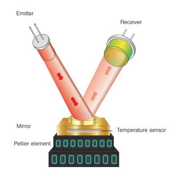
In order to ensure that any contamination (dust/powder particles) present on the mirror surface does not influence the measurement, the sensor checks the status of the mirror surface periodically. On start-up, the sensor goes into Digital Contamination Control Mode (DCC) where it heats the mirror surface until all condensation present on it evaporates and the mirror surface including any remaining contaminant particles is then taken as the reference.
