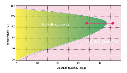
Accurate humidity measurement and attention to variations in parameters like feed concentration and incoming air humidity is important. The process can move from non-sticky production to a sticky powder production if the production parameters are not controlled and adjusted.
