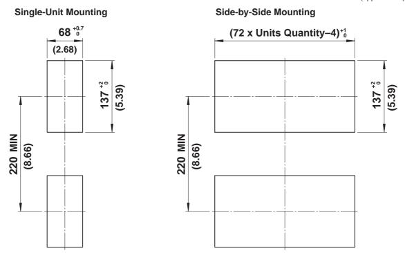
Note: If not specified, the tolerance is  $\pm 3\%$ . However, for dimensions less than 10 mm, the tolerance is  $\pm 0.3$  mm.
