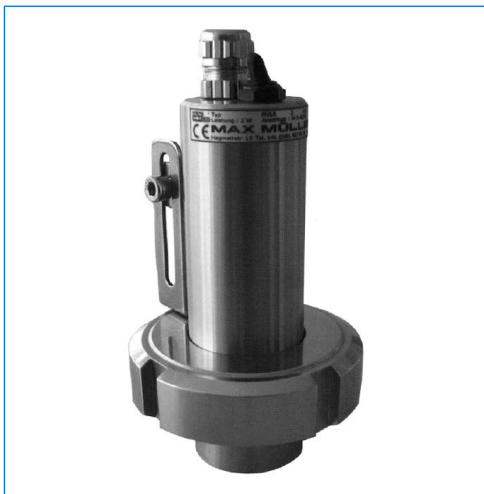
Micro LED light fitting, MVLR 2 LED E Sch1, 2 W, 24 V AC/DC, with integrated ON-OFF switch "E", mounted on VETROLUX screwed sightglass similar to DIN 11851, DN 32, PN 6
