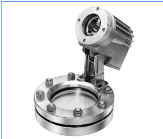
Type PEL 20 deH Sch, 230 V, 20 W, Ex d e IIC T6 Gb, Ex t IIC T80°C Db IP67, Ex II 2 G + D, mounted on circular sightglass to DIN 28120, DN 125, PN 10, in 1 port version
