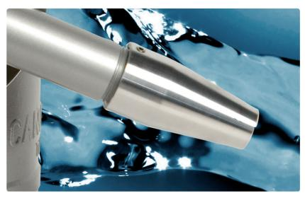
The SC 15TW is a 1.5" dual or four nozzle automated tank cleaning machine constructed of 316 stainless steel and other highly corrosion resistant materials. It has a fixed to moving gear ratio of 47 to 49 allowing it to produce a homogenous 360° pattern that is superior to that of any other rotating jet head in it's class.
