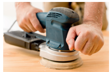
Orbital sanding of wood- and furniture boards
