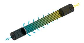
Compressed air, saturated with water vapor, flows through a bundle of tube-shaped hollow membrane fibers. A sweep orifice installed at the end of the bundle meters the amount of sweep air required to remove the water vapor from the dryer. Dry air then exits the tube bundle for use downstream. As long as the dried air isn't exposed to temperatures below the specified pressure dew point, no troublesome liquid water will form in the air system.
