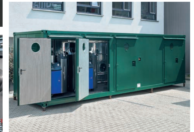
Fig.: Container steam system
