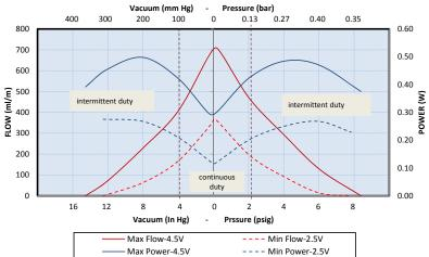
The above graphs represent examples of performance for the pumps series handling air at 800 feet (244M) above sea level at 75° F (24° C). Performance will vary depending on barometric pressure and media temperature. Curves are representative of standard pump configurations. Pump configurations could be customized for higher or lower flows, depending on specific customer requirements.
