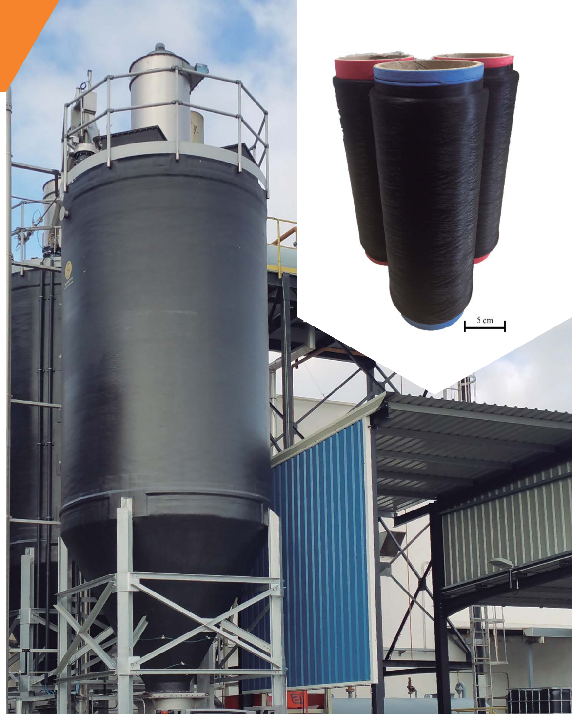
Image of an ATEX tank formulated with polyester resin and ACPS high Solid, and filament of conducting PET with avanPLAT 2
