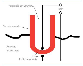
To measure the oxygen content, Nernst's equation (1) is used where  $PO_2(X)$  is the oxygen pressure which is to be measured.  $PO_2(REF)$  is the reference pressure which in this case is 0.209 as the reference gas is represented by the ambient air. T is the absolute temperature in Kelvin and C1 and C2 are constants.
