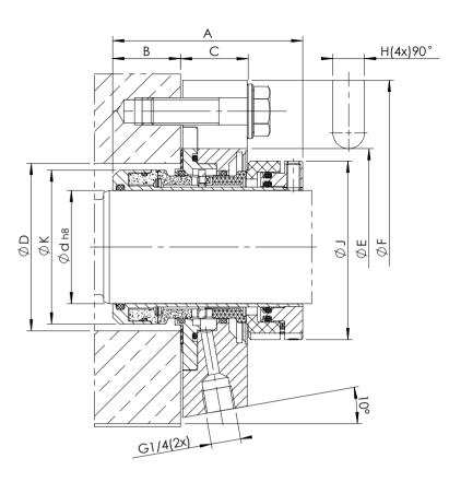
Max inside flush pressure = 12 bar Pmax = 25 barg Tmax = 200°C Vmax = 18 m/s (3600 rpm) Axial movement: ±2,0 mm
