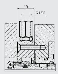
The axial built-in measurement increases with 19 mm irrespective of the shaft dimension.
