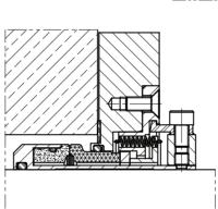
Pmax = 25 bar Tmax = 100°C Vmax = 18 m/s (3600 rpm) Axial movement: ±2,0 mm
