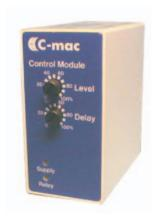
C-mac<sup>®</sup> current monitoring relay, type RC30, and voltage monitoring relay, type RV30 are universal metering relays, each supplied with 3 metering ranges, automatic detection of AC or DC input signal, plus a 24 VDC output voltage, for the supply of external sensors or the like.
