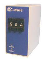
C-mac® module type RD53 is a digital pulse counter module, selectable as pulse divider or preselection relay. The pulse inputs can be activated from a mechanical contact, a transistor or a NAMUR sensor, and the reset input can be activated from a mechanical contact or a transistor. The unit is supplied with a "slave" transistor output, in this way several units can be connected to the same pulse
