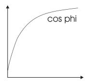
The phase angle between current and voltage  $(\cos \phi)$  is changing a lot between 0 and 60% load, therefore it is an advantage to monitor the phase angle if you want an alarm in connection with underload, f.inst. breakage of belts, pumps running dry, blocking of filters, etc.
