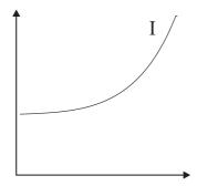
The current consumption of a motor is almost the same from 0 to 50% load, and after that it will increase with increasing load.
