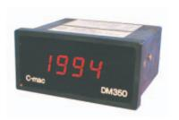
DM350 is a universal 3½-digit panel instrument with analogue inputs. The instrument has an adjustable display range between -1999 og +1999. The instrument can be used in connection with all C-mac® converters and relays with analogue outputs.
