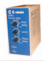
C-mac<sup>®</sup> module type RP91 is used for power monitoring of 1-phase and symmetrical 3-phase loads, f.inst. motors. RP91 can be connected directly to loads with nominal current consumption up to 6 A; If the current is bigger, a standard current transformer is used.
