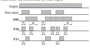
4: Special functions, controlled by start input and supply
