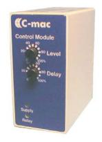
C-mac® monitoring relay, type RM34, is used for temperature metering in conjunction with Pt100 temperature sensors according to DIN 43760. A 3-wire metering principle is used, which means that the module compensates for the external cable resistance. The cable monitoring circuit also ensures that the relay will release in case of short-circuit or cable breakage.
