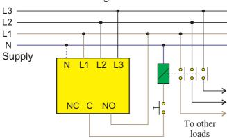
When the monitoring relay is connected as shown on the drawing above, the mains supply must be correct, before the load can be activated. This is particularly important if the load is sensitive to under- or over-voltage, and to ensure correct rotation direction of motors. This monitoring principle is recommended, when you want a general monitoring of the mains supply to several loads at the same time.
