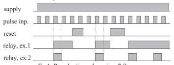
Ex.1: Preselection relay, pins 7-9 open Ex.2: Pulse dividing relay, pins 7-9 connected
