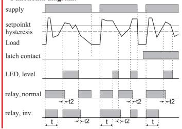
t =selected start-up delay, t2 =reaction delay
