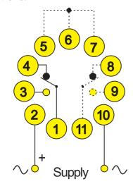
pin 8-9-11: 2-pole version only pin 5-7: reaction delay pin 6-7: nominal frequency
