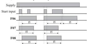
3: Delay on and interval, controlled by start input
