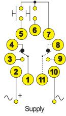
If you use transistor activation instead of contact, the emitter must be connected to pin 7.
