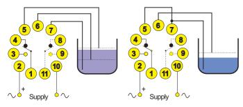
Example 1: 2 electrodes (max. and min. level)
