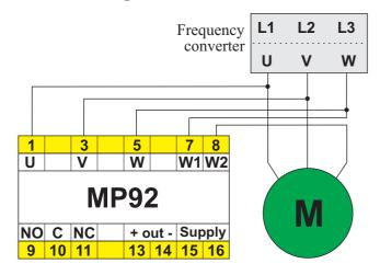
Supply voltage 24 VAC/DC is connected on pins 15-16. Output signal 0-10 VDC on pins 13-14.
