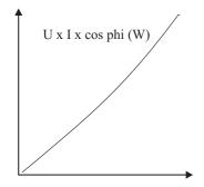
With power monitoring you can monitor all variables (supply voltage, current and phase angle), ensuring a very high sensitivity to even very small load changes, making this principle preferable for both over- and underload monitoring.
