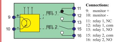
Converters with relay output are always supplied with input signal monitor.
