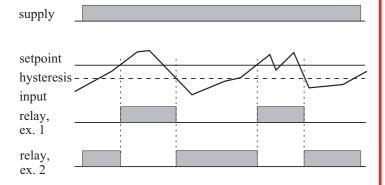
Example 1, undercurrent/voltage monitoring pin 6-7 not connected
