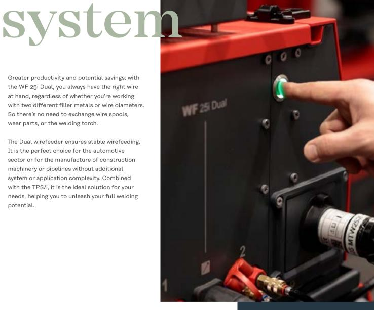
The illuminated LED indicator shows the welder which process line is currently active.
