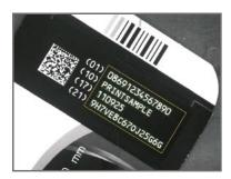
Rotation tolerant print inspection and incremental number check
