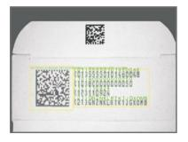
Track & Trace application with verification of GS1-Data Matrix and human readable text consistency (same data content), with additional Data Matrix quality inspection in accordance to ISO 15415
