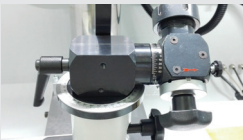
Item No. 16050 Precision grinding head ER32 with indexing, 19 mm chuck and laser adjustment
