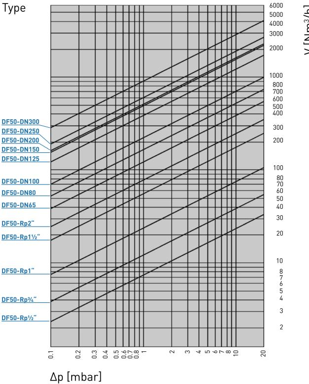
If the flow read from the diagram is based on the operating pressure instead of the standard conditions, the pressure drop read from the diagram must be multiplied by the factor: (1+ relative pressure in bar)
