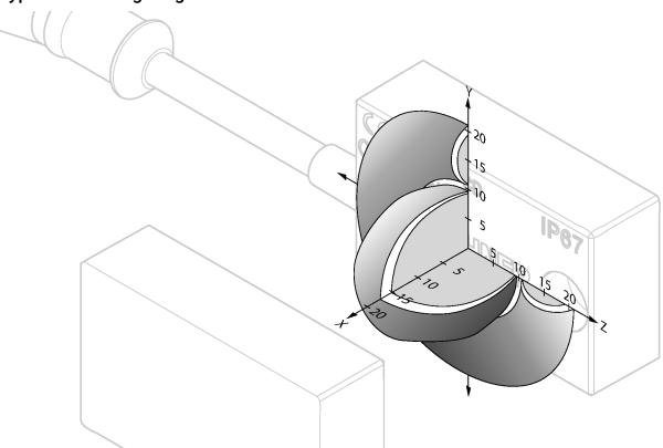
For a side approach direction for the actuator and read head, a minimum distance of s = 3 mm must be maintained so that the actuating range of the side lobes is not entered.
