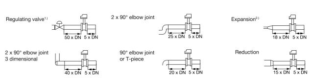
1.) If the valve cannot be mounted after the measuring device, the minimal distances have to be respected.
