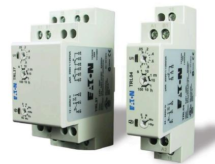
Eaton's Universal TR Series timers are a versatile and cost-competitive family of timing relays. The compact IEC-style housing installs easily onto a standard DIN rail, and the direct-wire design eliminates the need for additional sockets and accessories. Each timer has multiple user-selectable timing functions and timing ranges, and a universal input voltage of either 12 or 24 V to 240 Vac or Vdc, depending on the model.
