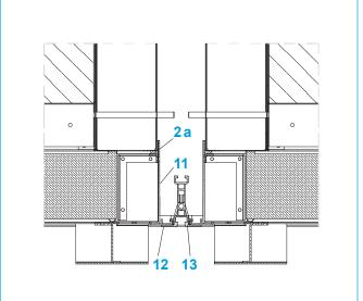
Fig. 2.2 Installation step 2: Lift filter cell in filter frame with FFU-IRC housing, Insert bearing rails 12 into grid ceiling UFR 55/70-T and lower the filter cell and FFU-IRC housing onto the bearing rails
