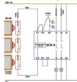
Three switches connected in series to an SCR-2 or SCR-3 to give Single Channel guard monitoring but with monitored Manual Start and Contactor Feedback check. Allows minimal wiring but higher current switching to K1 and K2 contactors.
