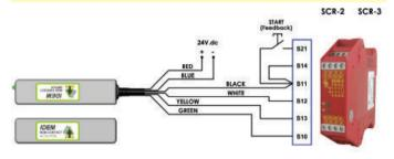
One switch connected to an SCR-2 or SCR-3 to give Dual Channel monitoring with Manual Start.
