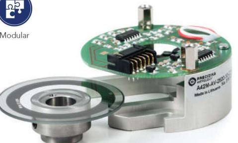
Photoelectric modular rotary encoder A42M is of incremental type and provides up to 25.000 output pulses per revolution. The absence of bearings and lubricants makes the encoder suitable for
