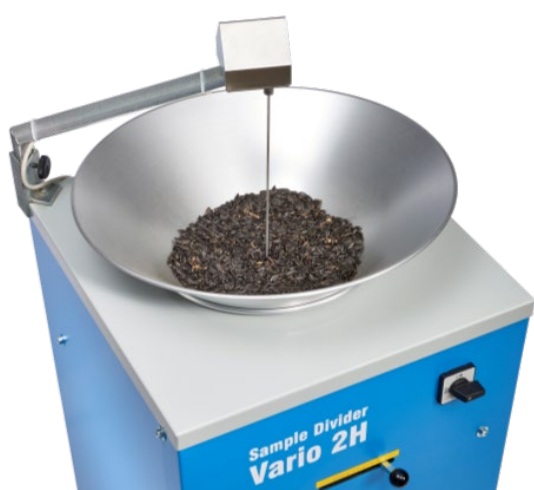
Figure 6: Agitator and mounting of the holder on the cover
