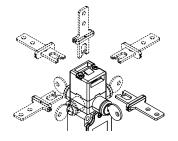
The head can be quickly rotated on each of the 4 sides of the switch by unfastening the two fixing screws. The release device can be rotated in 90° steps as well. This enables the switch to assume 32 different configurations.
